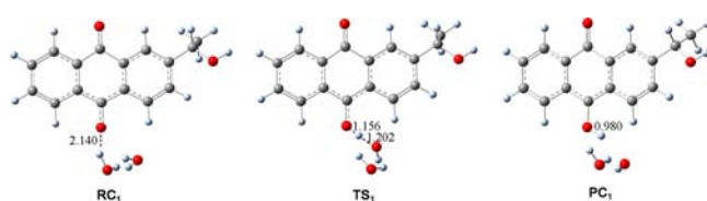
Figure 10. Optimized geometries of RC 1 , TS 1 , and PC 1 obtained from (U)B3LYP/6-31G* calculations for the protonation reaction of (2-HEAQ) 3 with H 2 O. Selected interatomic distances (Angstroms) are labeled.
